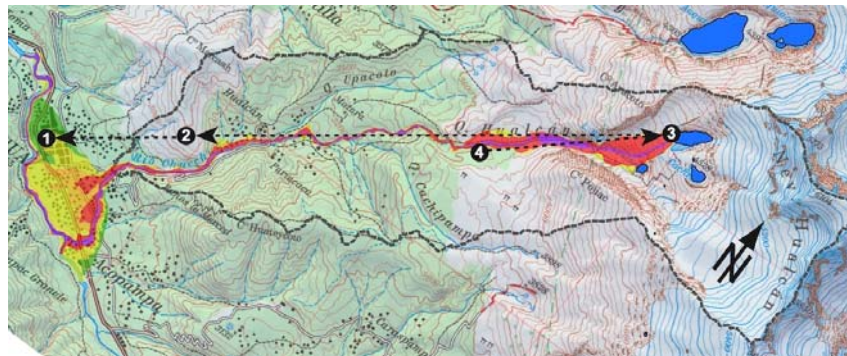
Figure 5: The four stations of the EWS. Dashed arrows indicate the direction of the signal transfer; the dashed line corresponds to the catchment margins. Background: topographic map from the Austrian Alpenverein and the GLOF hazard map.
