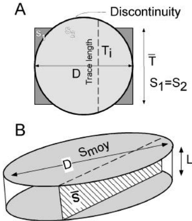
**Fig. 3** A) Relationship between the mean trace of the discontinuity set and its diameter, assuming a circular shape. B) Mean geometrical characteristics of the discontinuities.
