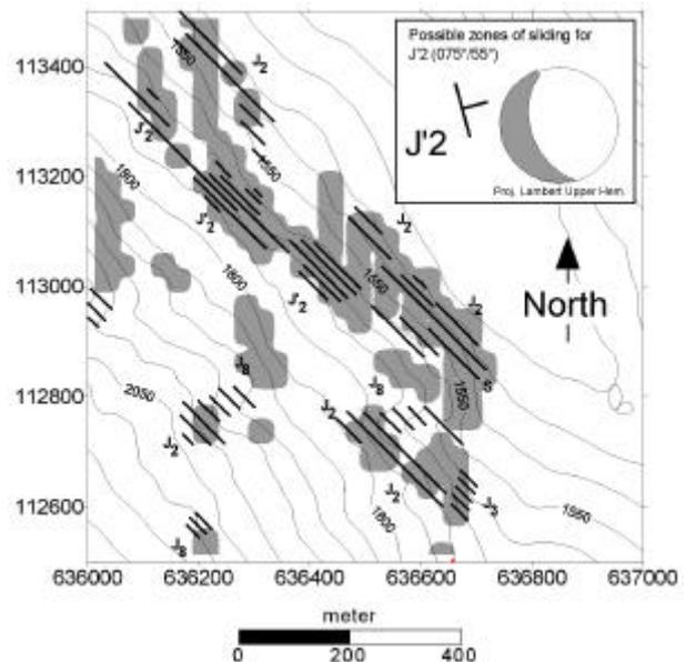
**Fig. 5** The shaded area represents the topographic part where the discontinuity set J'2 ( $075^\circ/55^\circ$ ) could induce rock sliding. The black lines indicate the observed rockfall activity produced by rock sliding on discontinuities. J'2 set has the same orientation but is slightly steeper than J'2 set. This area is the central southern part of the Fig. 4 (topographic data are used with the authorisation of the federal topographic office).
