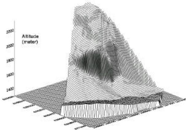
**Fig. 8** 3D representation of the Randa rockfall area before the disaster. The grey scale indicates a slip direction equivalent to the present slip direction ( $140^\circ/30^\circ$ ) measured in the upper part of the scar. This indicates that such movements could have produced rockfall. See text for explanation.
