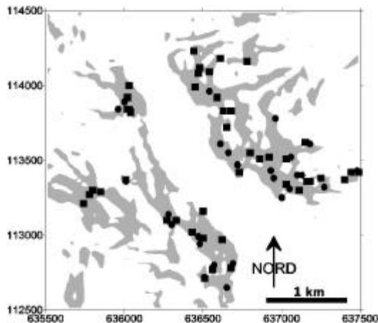
**Fig. 4** Map of the slopes steeper than  $50^\circ$  in an area of the Saastal in Switzerland (after <sup>7)</sup>). The majority of the rock instabilities are located within the steepest slopes areas. Squares are scars of past rockfalls and circles are observed present rock instabilities (topographic data are used with the authorisation of the federal topographic office).
