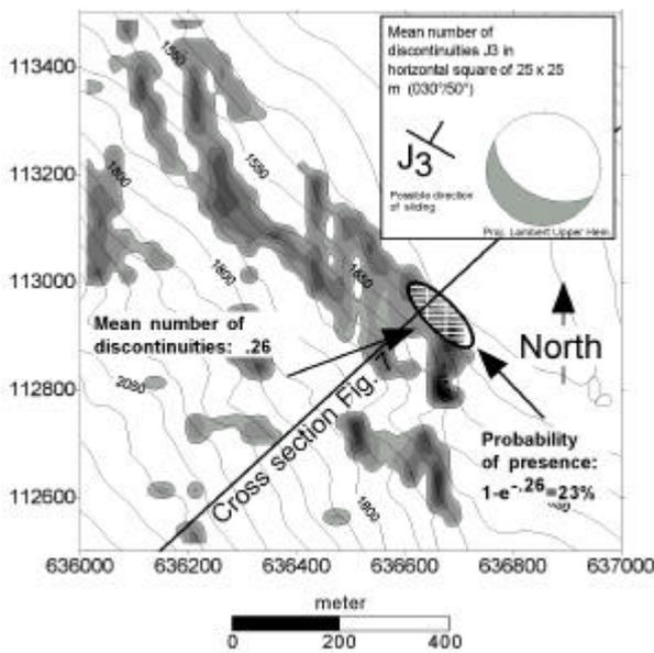
**Fig.6** The grey scale represents the calculated mean number of discontinuities J3 (030°/50°) that could be found on the topographic surface and could induce rock sliding. The mean trace length is 220m and the mean spacing 100m. This area is the central southern part of the Fig. 4 (topographic data are used with the authorisation of the federal topographic office).
